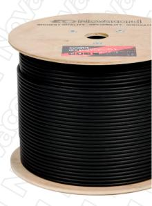
Star Quad multichannel snake cable, designed for all fixed audio installations. Each four conductor channel is completely isolated and contains Kevlar 29 for tensile pulling strength. We use large numbers of thin wire strands in the copper conductors and overall braided shield. Cable designed to avoid the release of toxic matter in case of fire, because they do not contain any halogens.
