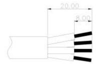
(3) Insert the cable conductor part into the inner core terminal and locked with 0.5 Nm torque screws.
