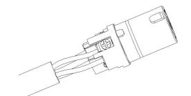
(4) Push the cable clamp and inner core assembly into the housing.
